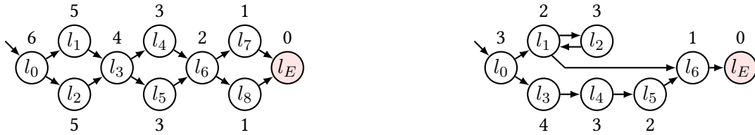
(a) Example where BFS would need an exponential number of steps to reach l_E .
